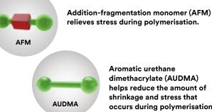
Aromatic urethane dimethacrylate (AUDMA) helps reduce the amount of shrinkage and stress that occurs during polymerisation.
